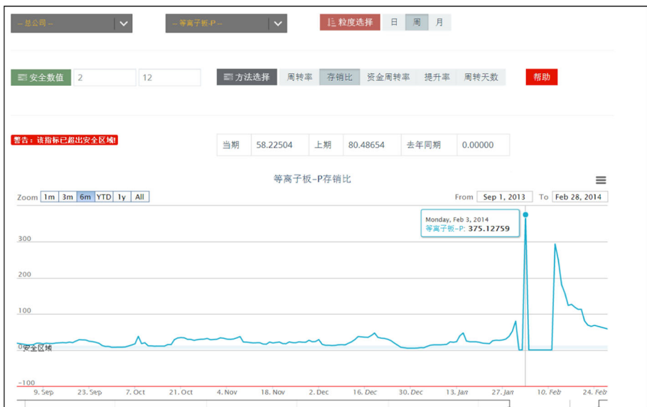
Fig. 25 An example of anomaly detection is illustrated. The normal value range is set for the time series. An anomaly is detected if the value falls out of the normal value range
